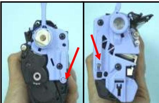
6. Assemble the hopper and waste section by inserting the Plastic pivot pin and Metal Pivot pin as shown in the photo.
