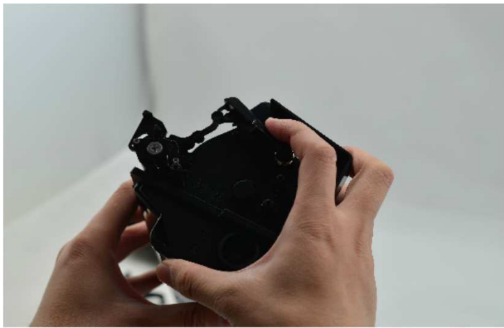
37 / Completed installation the toner outlet cover
