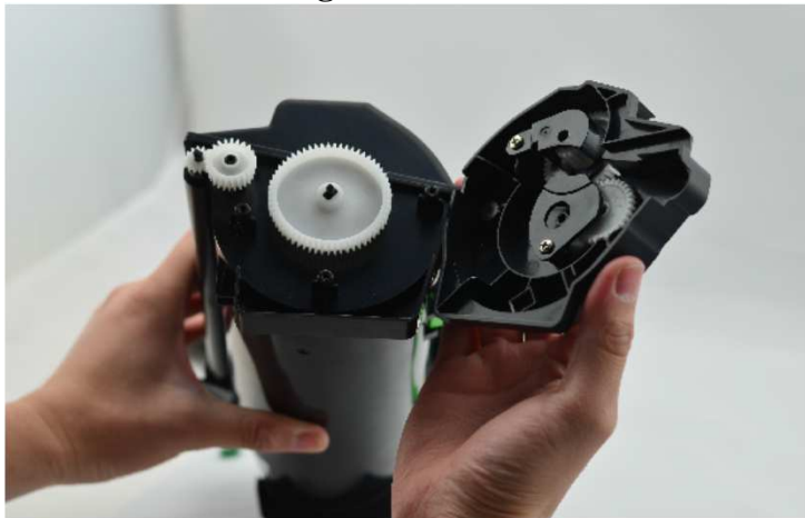
21 / Set down the agitator gear and cover
