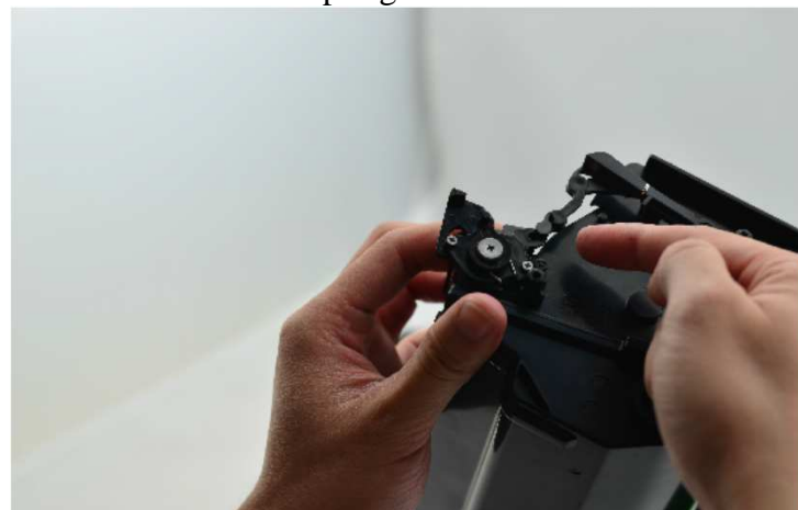
36 / Fixing the toner outlet cover
