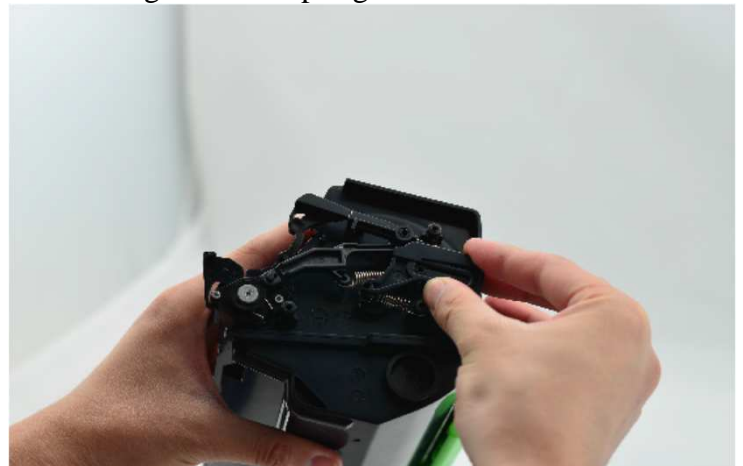
44 / Link spring and drive sliding
