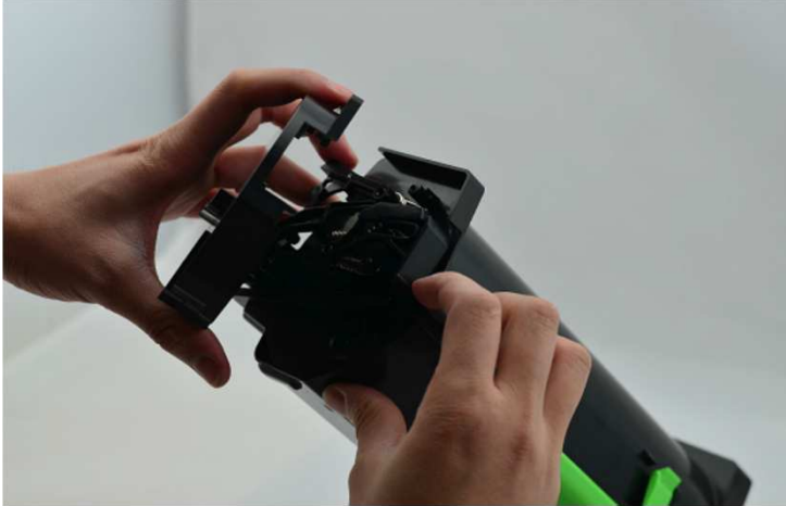
71 / Install the right end cap ( push on trigger )
