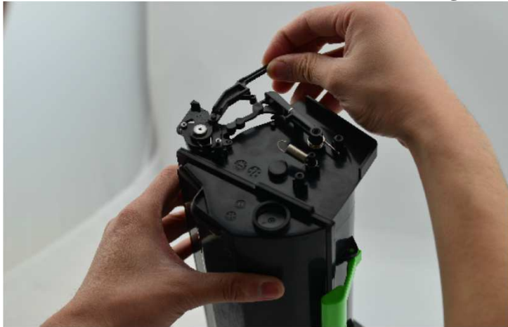
41 / Install the drive spring and drive linkage
