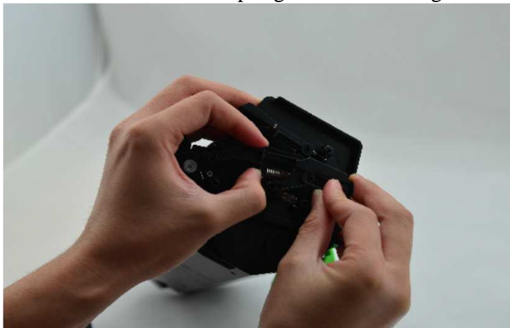
45 / Link the drive linkage and drive sliding
