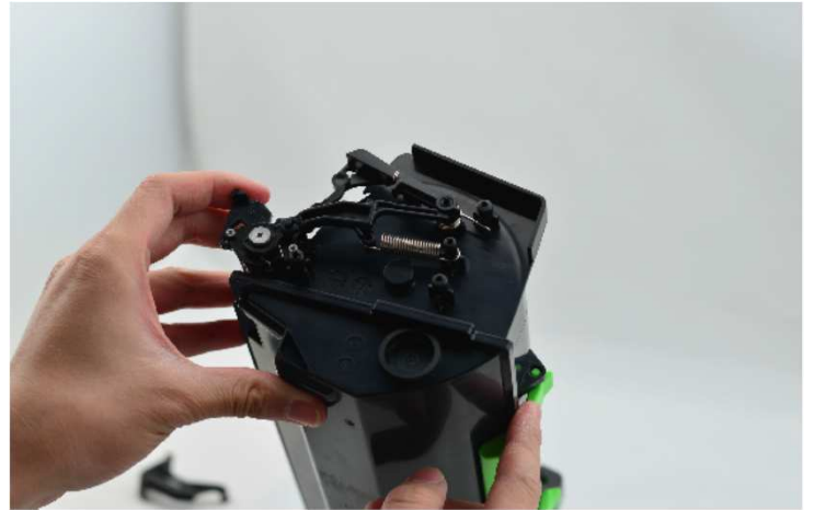
42 / Fixing the drive spring
