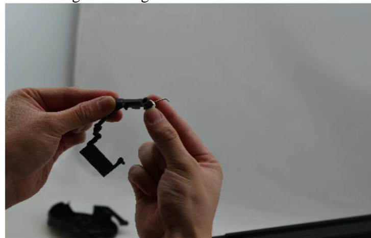
34 / Install the drive spring
