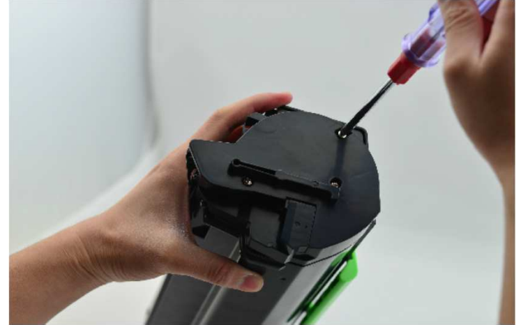
72 / Lock that end cap by fixing 3 screws
