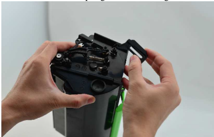
43 / Install another drive spring and drive sliding
